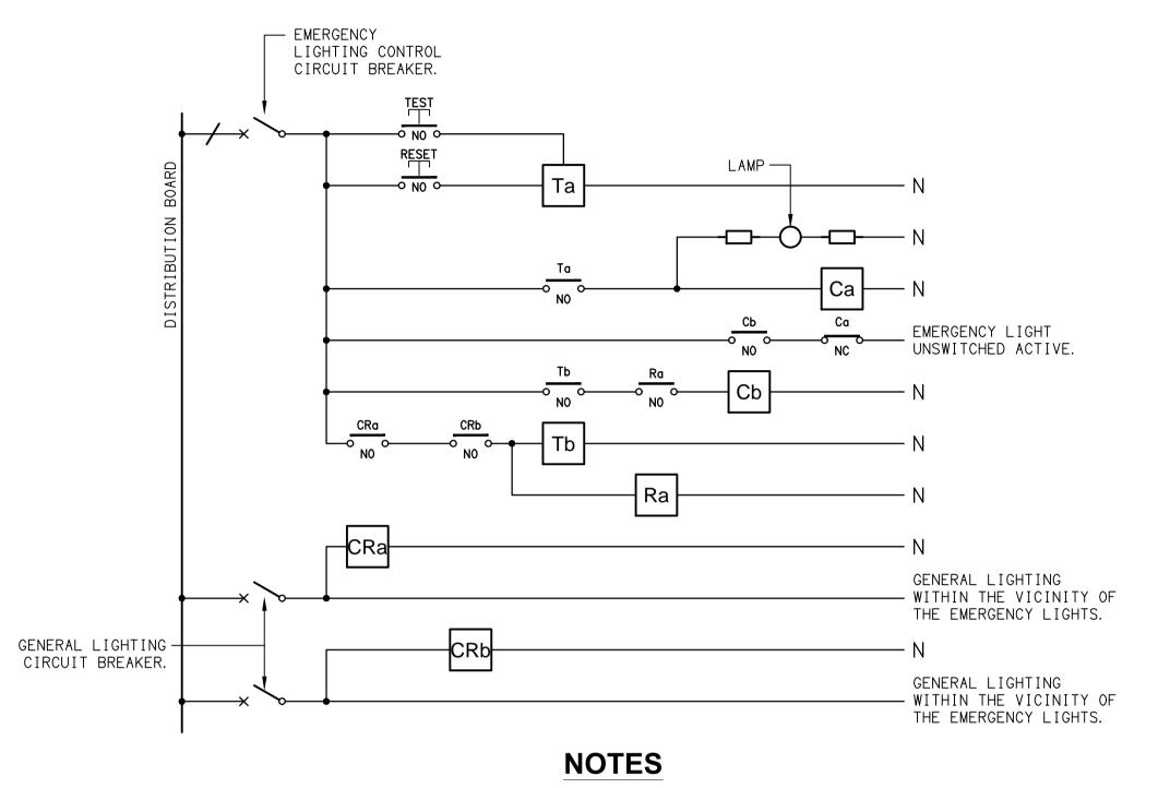
**SCHEMATIC EMERGENCY LIGHTING**  1. THE EMERGENCY LIGHT UNSWITCHED ACTIVE / GENERAL LIGHTING SWITCHED ACTIVE CIRCUIT ARRANGEMENT AND CONTROL IS TYPICAL FOR ALL CIRCUITS SUPPLYING EMERGENCY LIGHTS.
